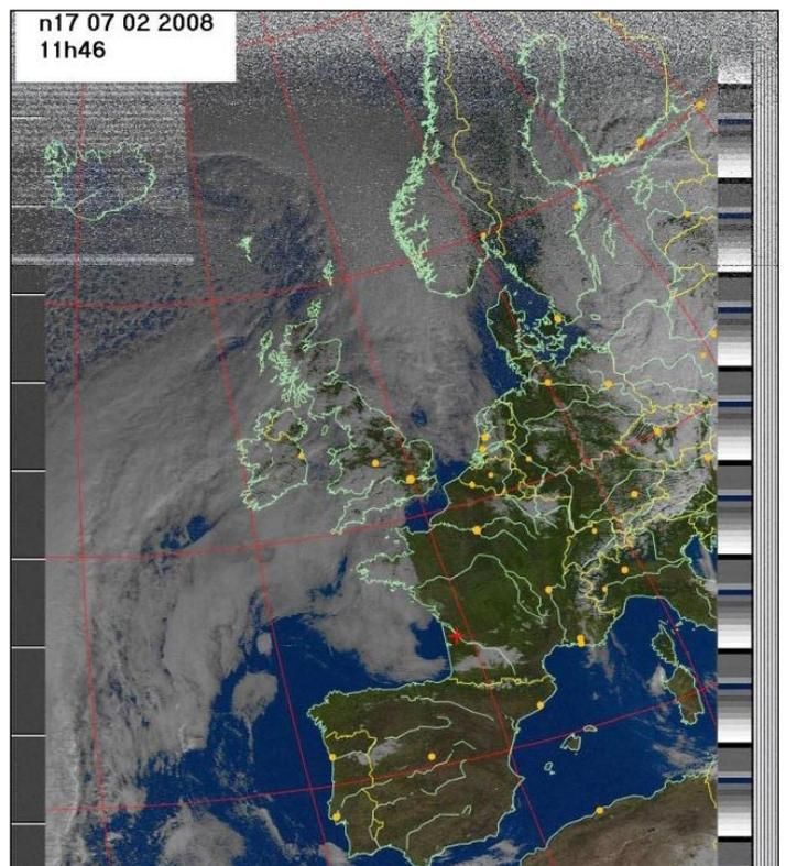
Figure 6 - Orbcomm satellite interference
