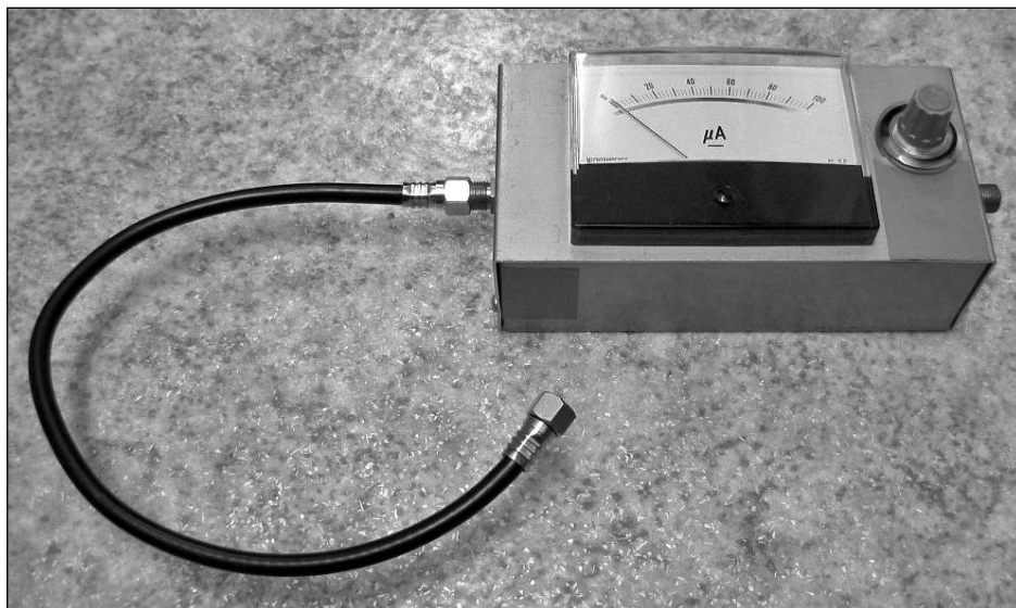
The author's completed satellite signal meter
